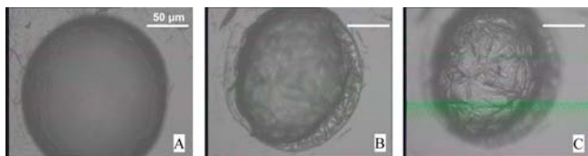
Figure 4. Light microscope images showing the age-induced shrinking effects for air bubbles stabilized by C_b = 10^{-2} wt % HFBII. Image A shows a freshly produced bubble, with the focusing level exactly at the A–W interface. Images B and C show the same bubble as in image A after 4 days of aging under atmospheric pressure, with the focusing level at the A–W interface and slightly above the interface, respectively. The size bar = 50 \mu\text{m} .
